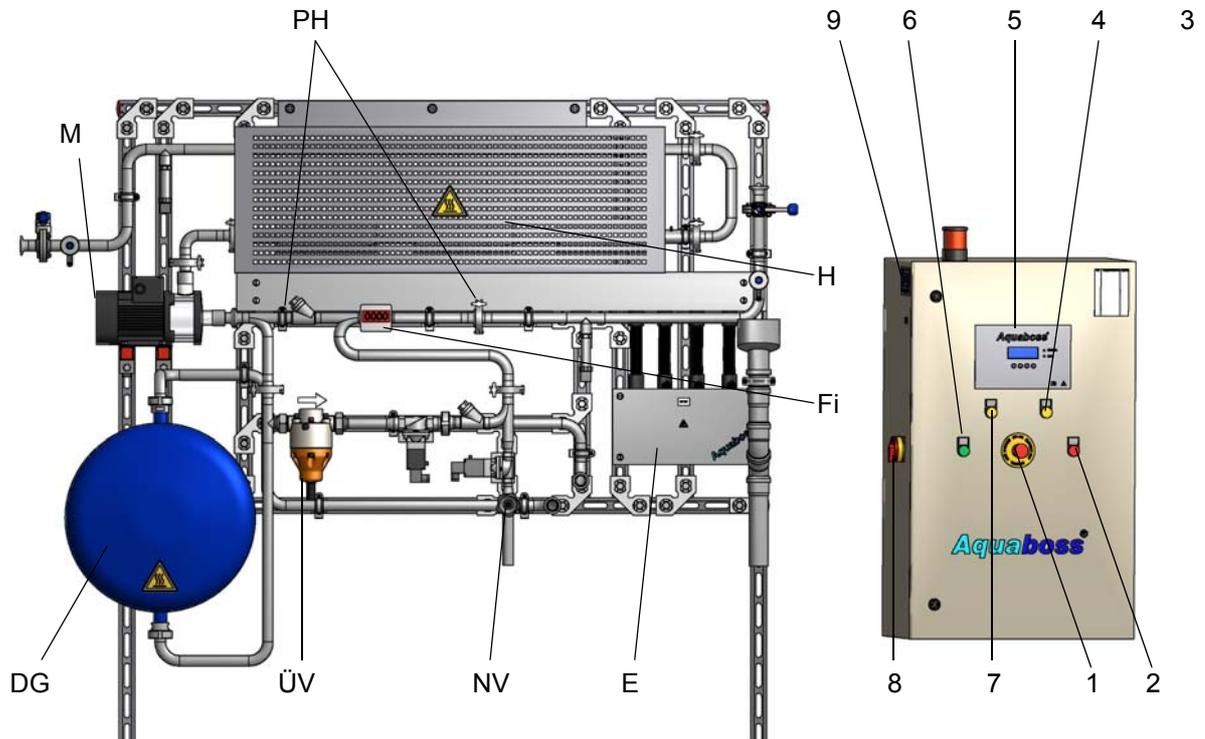
Figure 6-3: **Aquaboss® Hot Rinse SMART 10/20/30/40/50 front view**
