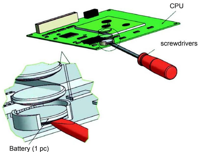
**Figure 8-5: Battery removal**
