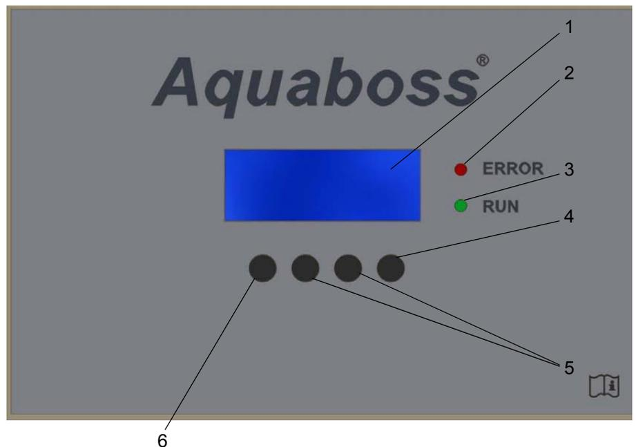
**Figure 7-4: Display with function keys**
