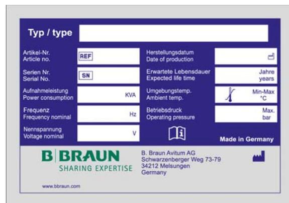
Figure 5-8: Example of a type plate
